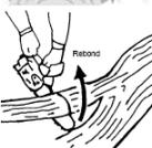
21. When cutting a limb that is under tension, be alert for spring back so that you will not be struck when the tension in the wood fibers is released.
