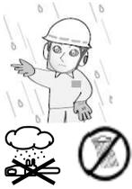
22. Do NOT expose to and do not use during bad weather conditions: Never cut in high wind, bad weather (e.g. rain, storm, snow...), when visibility is poor or in very high or low temperatures.
