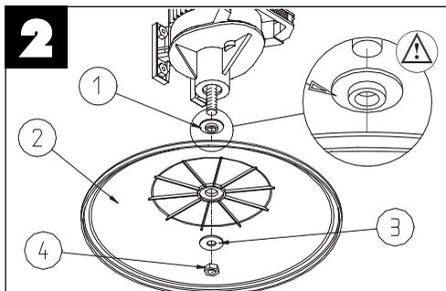
Screw the agitator tightly into the motor shaft.
