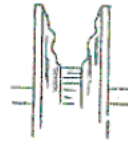
Extremely worn groove of pulley
